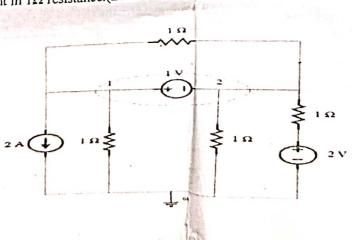
d) Find the current in all branches shown in figure using mesh analysis. (BKL > = K3 Level).
