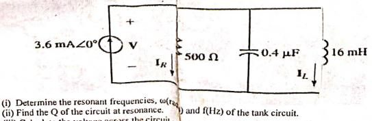
(iii) Calculate the voltage across the circuit a
